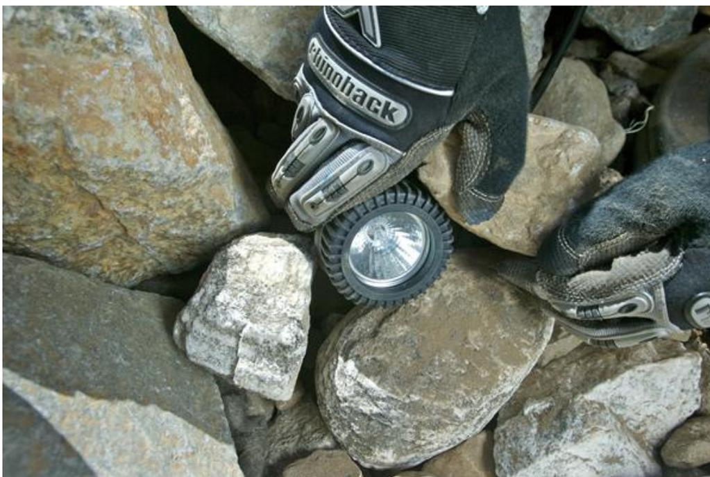
Try to place the light body in between two or more rocks pointing out. This will conceal the light from view during daylight hours. Lights at the base of the waterfall pointing up are popular and allow you to continue viewing the falling water after dark.
